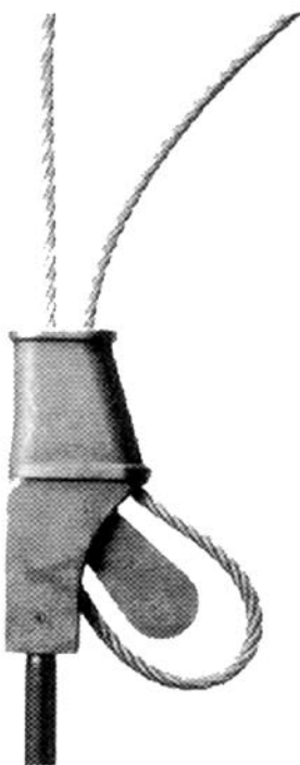
Figure 7: Place wedge in the loop, choosing the correct wedge for the socket
