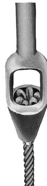
Figure 3: Turned ends pulled into basket ready for pouring
