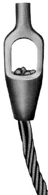
Figure 5: Incorrectly socketed wire rope showing loss of rope lay
